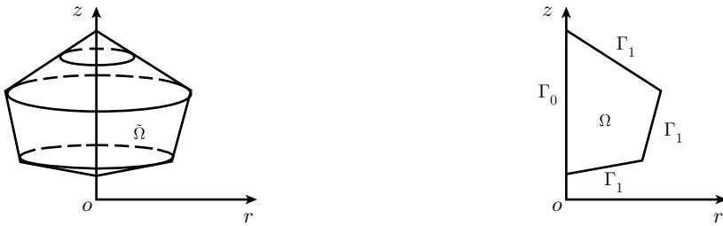
FIGURE 1. The 3D axisymmetric domain \tilde{\Omega} (left); the meridian polygonal domain \Omega (right).
